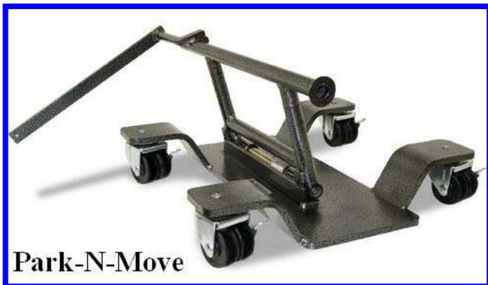
Although there are other products on the market that claim this ability, this item does it with a minimal footprint: 18" x 16" x 5"; weighing in at 33lbs, 3/8ths steel, powder coated and supporting up to 1,100 lbs of bike. The secret here is four 360 degree; caster type wheels each with 3 sets of ball bearings, two of which employ a locking device on the caster.
