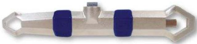
Each end of the wrench features a hexagonal head with an adjustable hydraulic piston slider to provide a three sided, full surface contact fitting with the bolt. Even works to extricate damaged, stripped and rounded-off bolts. Its hydrokinetic slider system is faster and easier to adjust to the proper size. Turn the valve located in the center of the wrench a quarter turn to release piston, which will adjust to bolt or nut diameter, and tighten for a firm, custom grip on every fastener.
